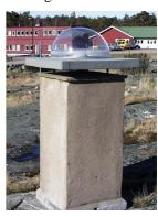
Figure 7: GPS antenna with radome at Onsala before and after February 1, 1999.
