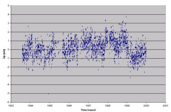
Figure 8: Coordinate time series (from the BIFROST project) of the up component at Onsala.
