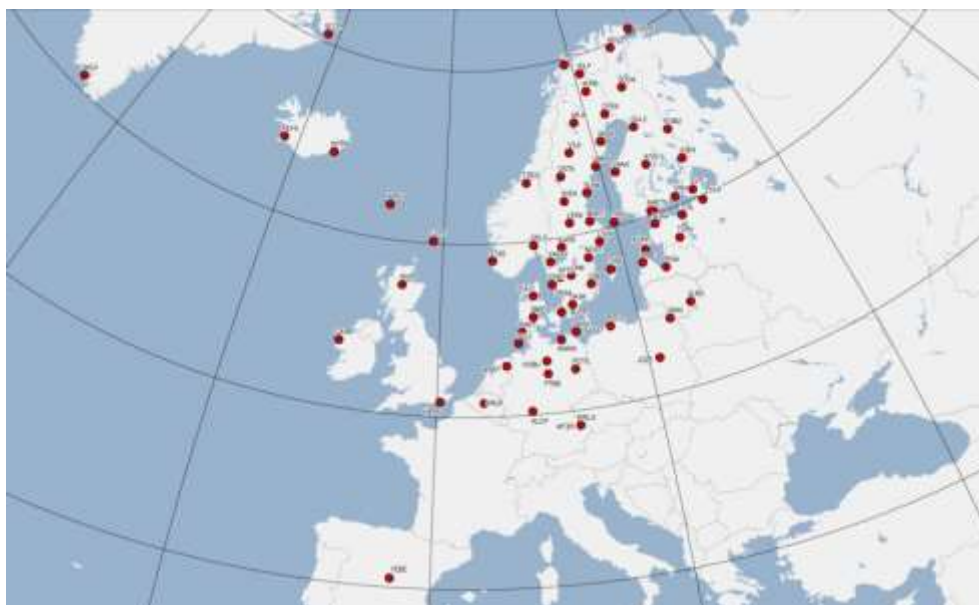
Figure 1.1: The NKG EPN AC sub-network of 88 permanent reference stations for GNSS. Source: www.epncb.oma.be .
