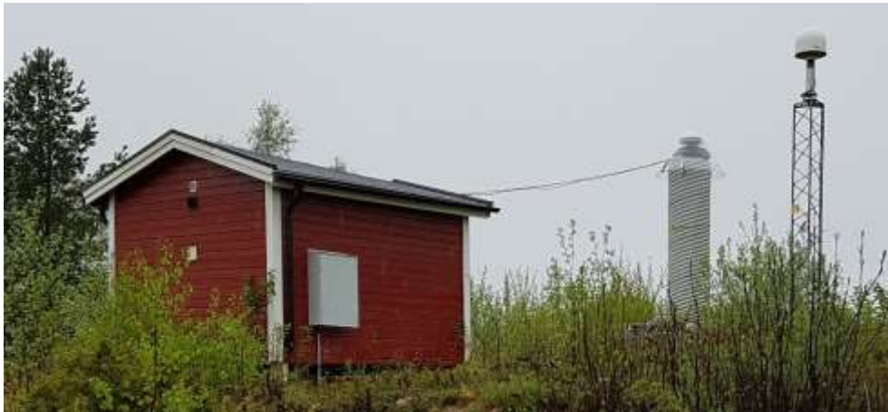
Figure 1.3: Sveg is a SWEPOS class A station. It has both a new monument (established in 2011) and an old monument (from 1993).
