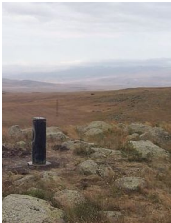
Figure 1.11: Amasia, one of the stations in the zero-order geodetic network of Armenia. The reference frame ARMREF 02 was ratified as a ETRS 89 realisation at the
