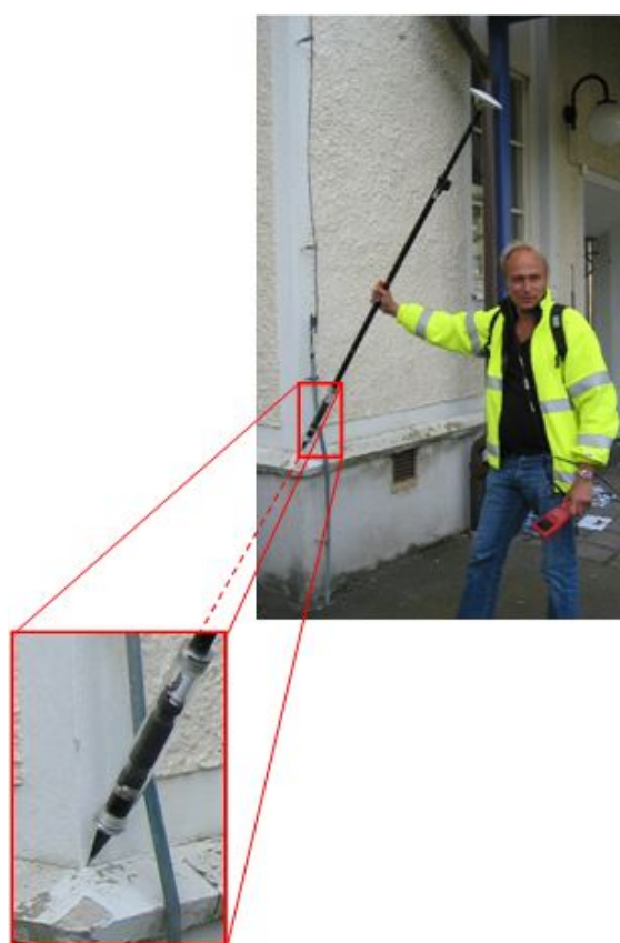
Figure 1.2: Demonstration of a combination of GPS in RTK mode and inertial technique.
