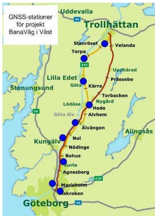
Fig. 2. Project adapted reference stations (blue dots) set up for an infrastructure project north of Gothenburg. The in-between-station distances are 10-15 km.
