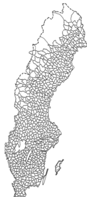
Figure 2: The levelling network realizing RH 2000.
