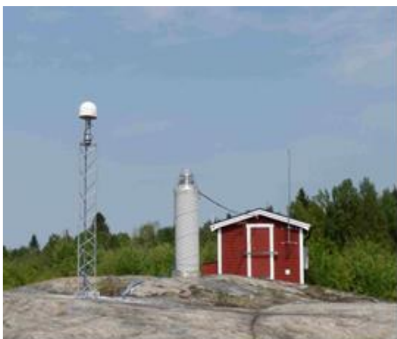
Figure 1.3: Hässleholm is one of the SWEPOS stations belonging to class A. It
