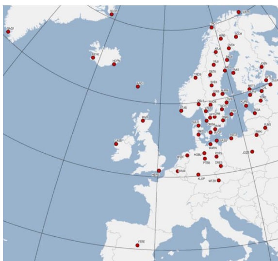
Figure 1.1: The NKG EPN LAC sub-network of 68 permanent reference stations for GNSS in January 2015. Source: www.epnch.oma.be .
