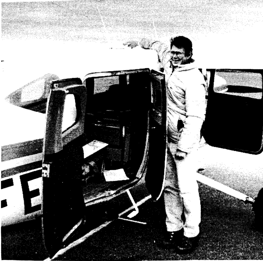
Figure 1. The Cessna aircraft with installed camera and GPS equipment.
