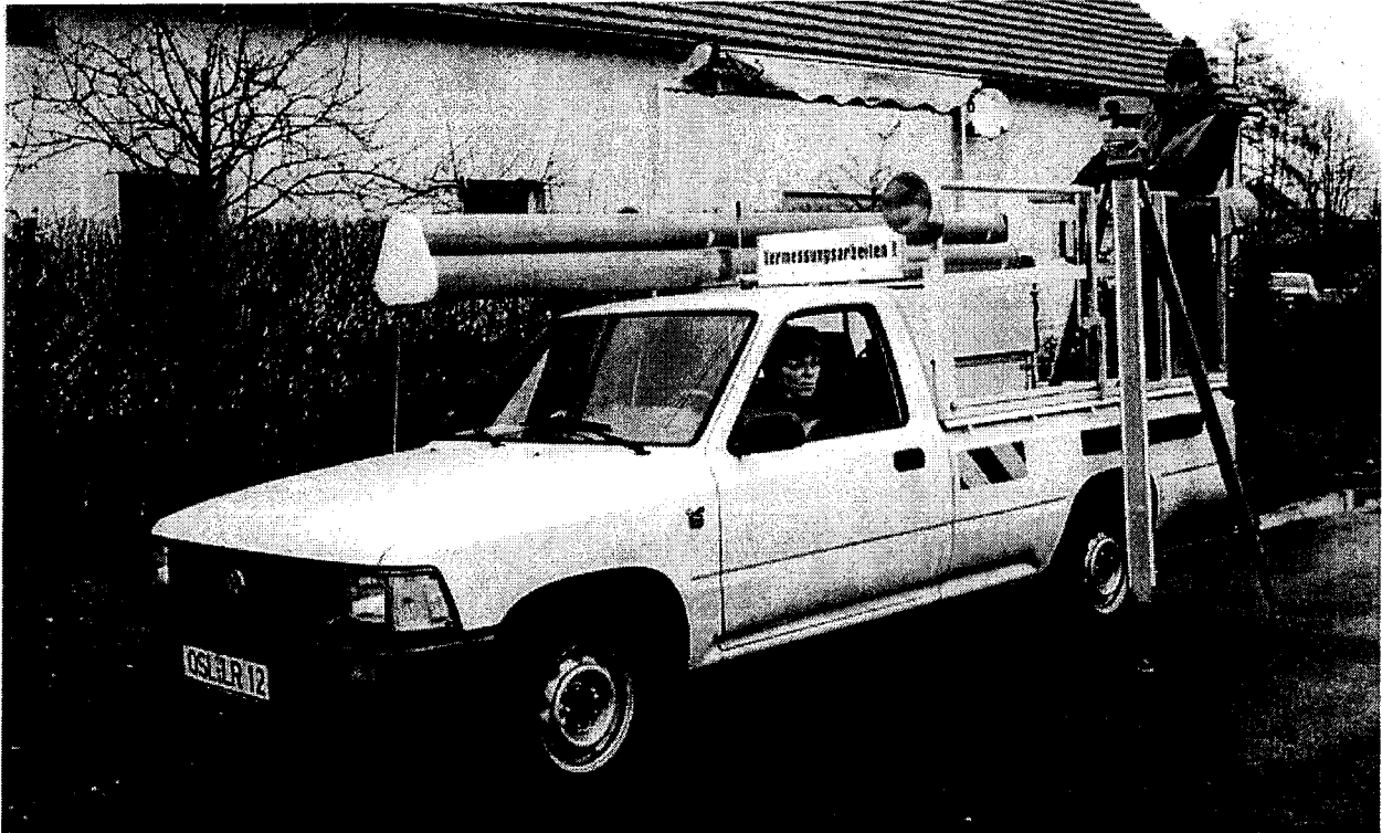
Figure 3: The instrument vehicle of the LAUBAG motorized levelling party
