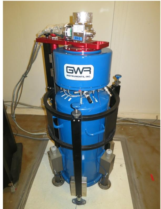
**Fig. 6.** New superconducting gravimeter OSG-073 of the FGI. Photo J. Näränen
