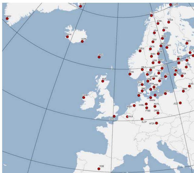
**Fig. 1.1.** The NKG EPN LAC sub-network of permanent reference stations for GNSS is concentrated to northern Europe (in May 2016 it consisted of 74 stations). Source: [www.epncb.oma.be](http://www.epncb.oma.be).
