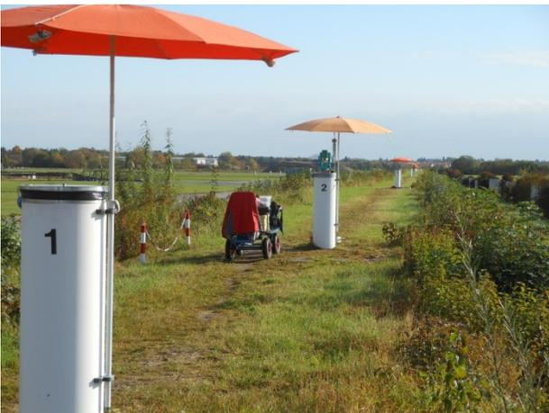
**Fig. 13.** The UniBW geodetic baseline near Munich is suitable for comparisons between GNSS and terrestrial measurements. The scale of also this baseline is now traceable to Nummela. Photo J. Jokela
