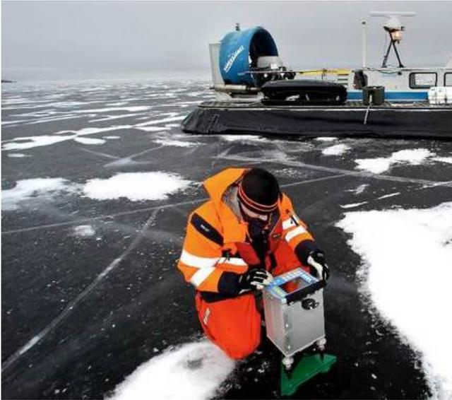
**Fig. 1.8.** Relative gravity measurements in March 2011 on Lake Vänern, the largest lake in Sweden. Photo: Mikael Lindblom.
