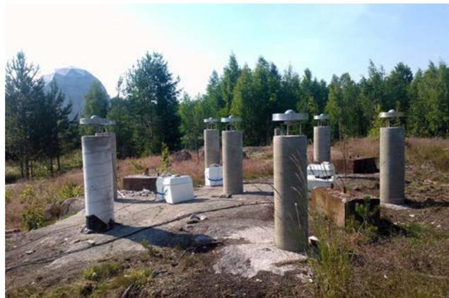
**Fig. 12.** GNSS antenna test field, “revolver”, at Metsähovi. Photo M. Poutanen
