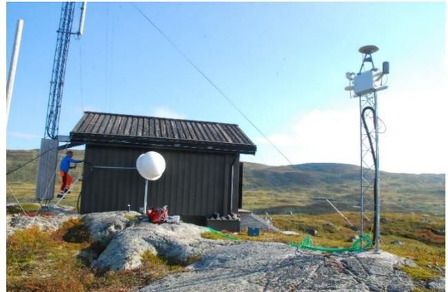
**Fig. 5-2** Installation of weather sensor – Haukeli station
