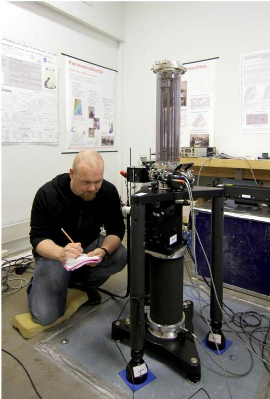
**Fig. 5.** Jyri Näränen is observing with the renewed absolute gravimeter FG5X-221. Photo M. Poutanen
