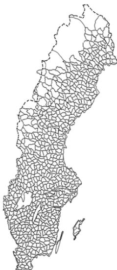
**Fig. 2.** Levelling lines of the third precise levelling of Sweden.
