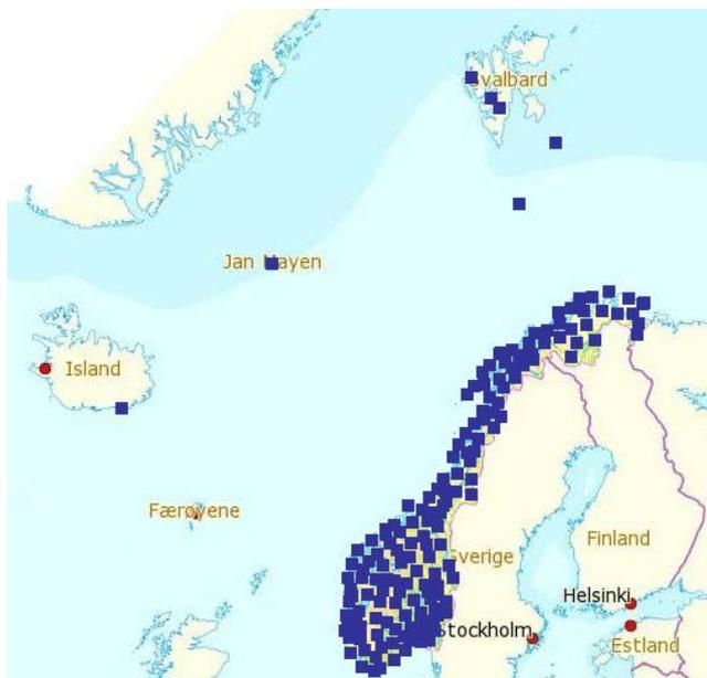
Figure 2-1 GNSS receiver network (1hz)
