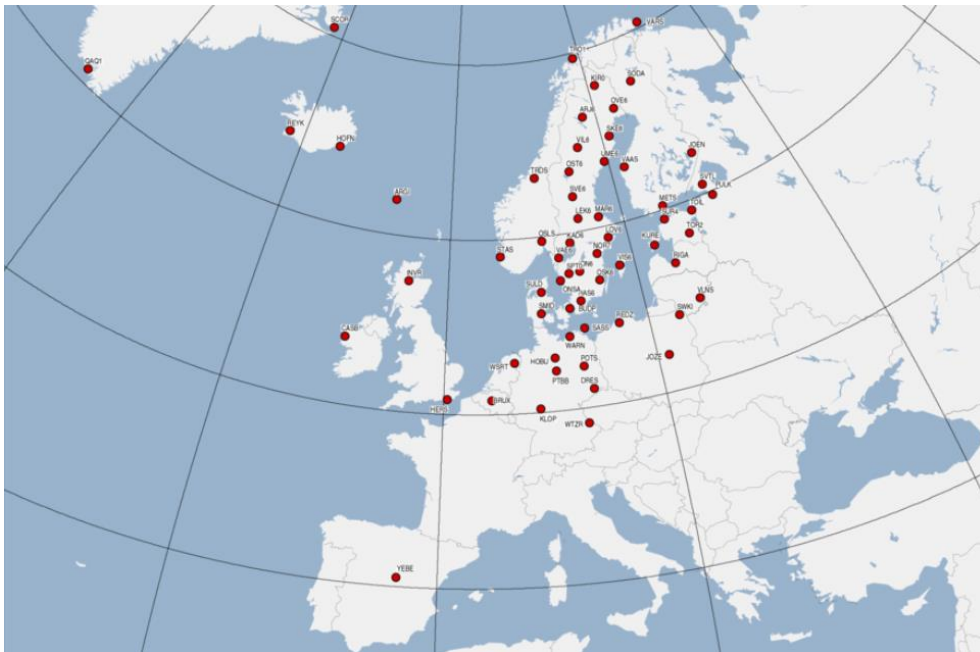
Figure 1.1: The NKG EPN LAC sub-network of 68 permanent reference stations for GNSS in January 2015. Source: www.epncb.oma.be .
