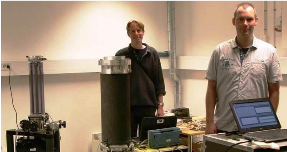
Figure 2.2: Calibration of the super-conducting gravimeter with two absolute gravimeters (both Micro-g LaCoste FG5) in May 2014.
