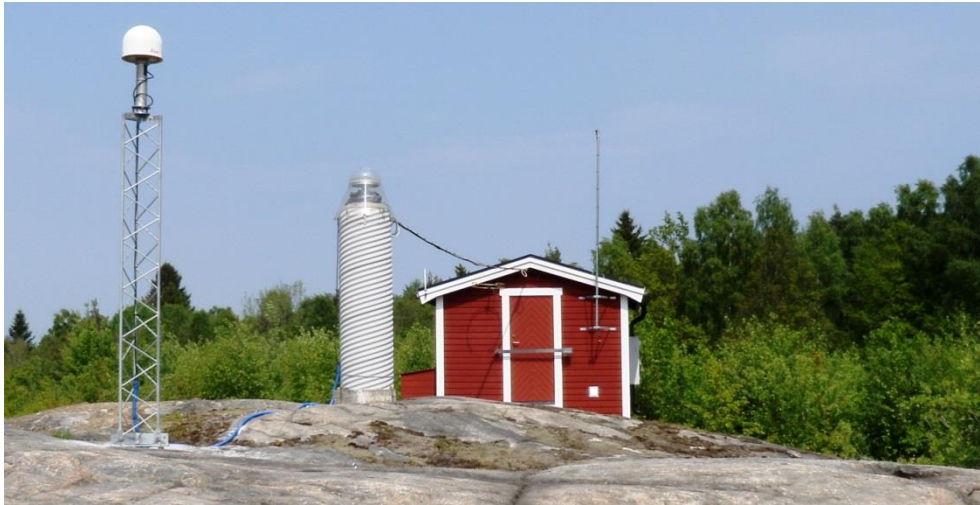
Figure 1.3: Hässleholm is one of the SWEPOS stations belonging to class A. It has both a new monument (established in 2011) and an old monument (from 1993).
