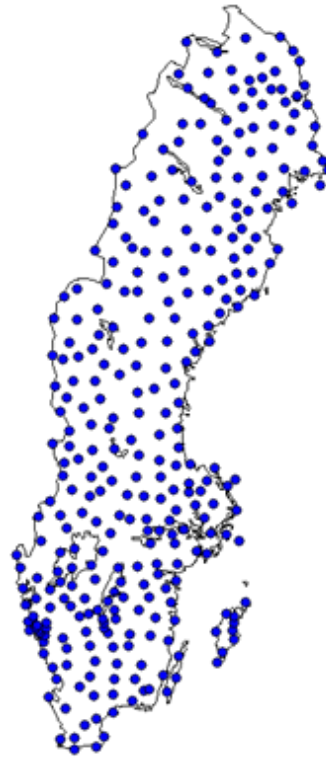
Figure 1.7: The approximately 300 SWEREF points from the RIX 95 project, which totally included 9029 points.
