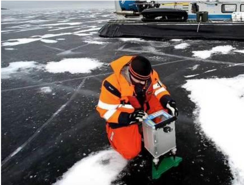
Figure 1.8: Relative gravity measurements in March 2011 on Lake Vänern, the largest lake in Sweden. Photo: Mikael Lindblom.
