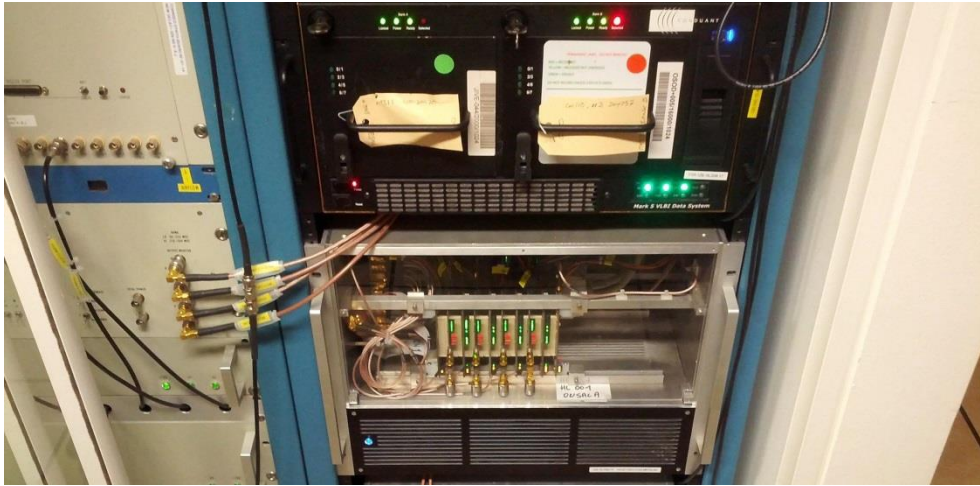
Figure 2.1: The new rack for VLBI at Onsala Space Observatory is a modern digital backend system.
