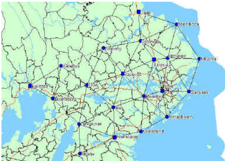
Figure 2.1: Network for one of the ongoing production projects with network RTK in the SWEPOS™ network of permanent reference stations.
