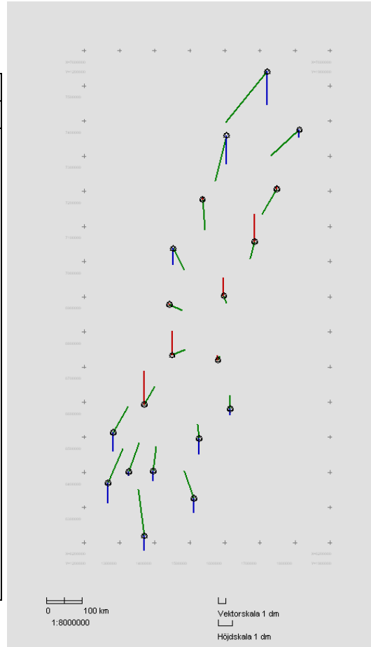
Figure 6: Residuals from fit with 3 translations and rotations around the topocentric z-, y- and x-axis. Green vectors for horizontal residuals and red/blue for vertical.
